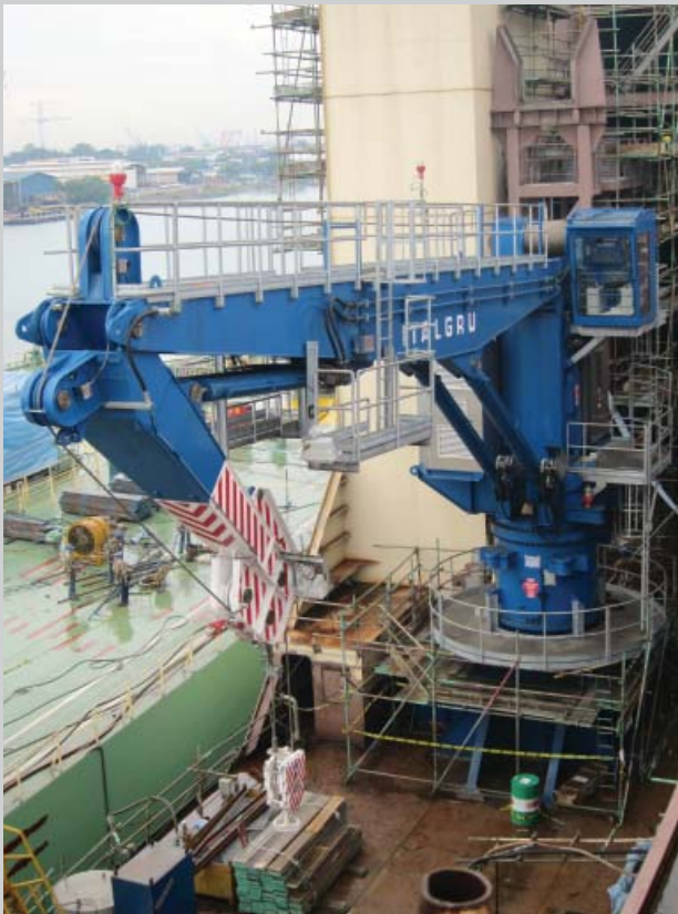
Knuckle Boom Crane Type TK 820 EH – Saipem – Castorone Pipe-Lay Vessel (- 40 Celsius)
