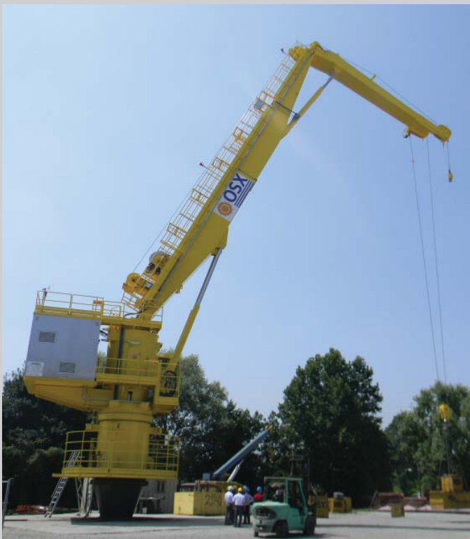
Knuckle Boom Type Pedestal Crane TK 1200 EH – SBM – OSX – FPSO OSX 2
