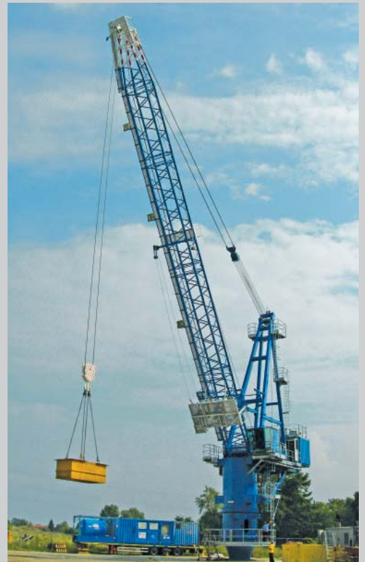
Lattice Boom Pedestal Crane Type TS 1200 E - Saipem - Castorone Pipe-Lay Vessel (-40°Celsius)
